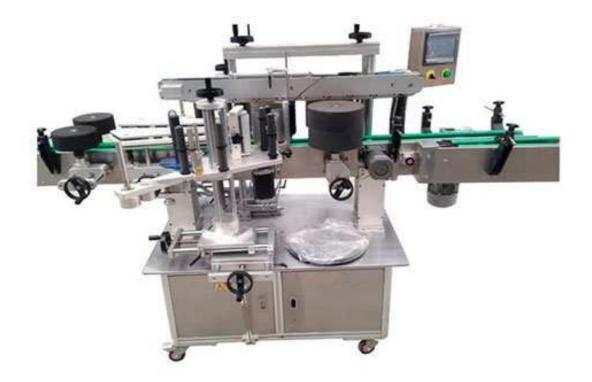
This series of products are not only suitable for the s round can/jar/cylinder/bottle but also flat square two sides bottles in pharmaceutical, pesticide, food & chemical industries.
