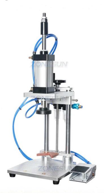
This desktop bottle cap-pressing machine is suitable for pressing cork, plastic lids, etc. Driven by high-quality cylinder, the machine can work stably, improving work efficiency. The pressing component can be customized according to caps' size. This machine is widely used in food, cosmetics, wine industries.
