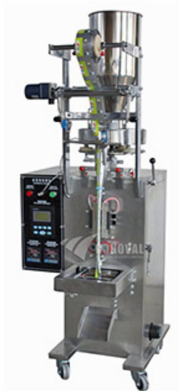
The integrated processes of bag making, measuring filling, sealing cutting, counting and hot pressing codes can be done automatically.
