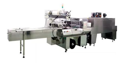
Hermetic Sealing with barrier shrinkable film and gas flushing for Modified Atmosphere Packaging (MAP) is an ideal wrapper for fresh fish packaging to achieve longer shelf life.
