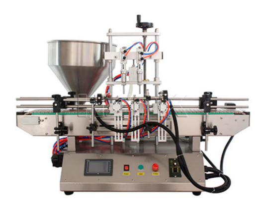
Tabletop paste filling machine is suitable for liquid product or paste product.
