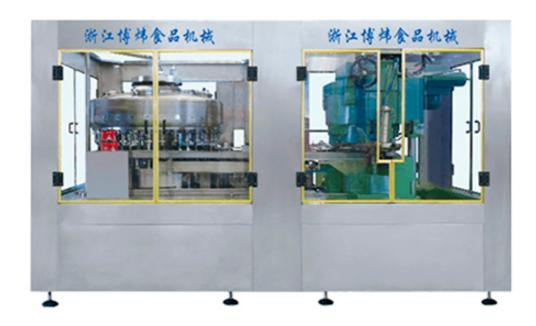
The machine is a device developed by Bowei machinery on the basis of digesting and absorbing domestic and international (still) pop can filling and seaming machines (sealing machines). It adopts the normal pressure filling principle.
