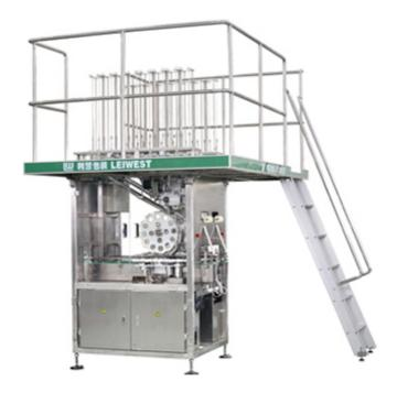
JGS-1 Cap Applicator is suitable to cap and put tableware (straw, spoon, small fork, etc.) on various round packaging containers. The machine uses modulized design and can be applied to containers of different sizes, such as cup, bowl and can, etc. It can also realize fast switching-over for different containers, with features of low power consumption, simple operation and convenient maintenance, etc.
