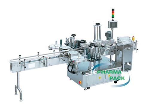
Designed for labelling flat bottles from two corner sides. This is a reliable, high performance machine, designed in conformance with current and proposed GMP. Production capacity is up to 200 bottles per minute. Conveyor height is 870  $\pm$ 30 mm. Applicable container size must be within  $30-200 \times 40-250$  mm.
