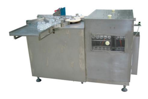
This machine is applied to clean the clinical bottle or oral liquid bottle with its revolving drum structure. Supply the bottle by feeding disk then transfer it through Wheel and input the bottle with revolving drum at interval. After passing through the ultrasonic water area, clean the bottle with recycling water (or tap water), distilled water and purified compressed air alternatively.
