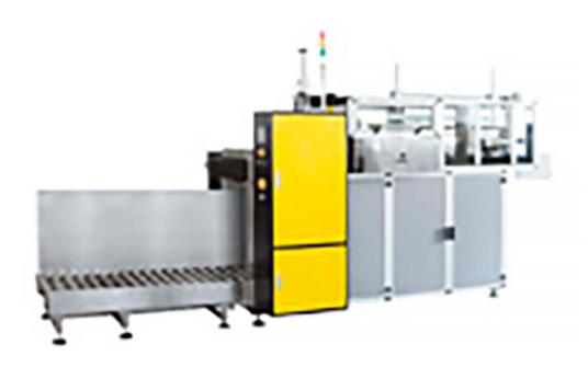
The Youngsun CF-30TB Carton Erector is an innovative new case erector that is capable of erecting and sealing cases with pressure-sensitive tape or hot-melt glue at speeds up to 25 cases per minute.
