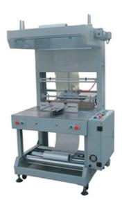
BSF-6030X semiautomatic sleeve sealing machine is a type of economic one among BSF series, simple operation, push the products manually or pneumatically, sealing the film and the products enter the shrink tunnel automatically, and used PE film to pack products.
