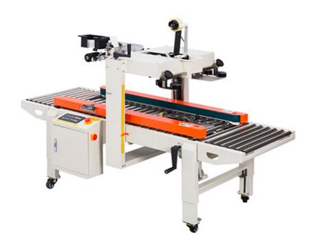
The machine uses instant adhesive tape to complete the upper and lower sealing of the box, and at the same time uses the folded sheet to complete the labeling. The sealing is firm, the labeling position is adjustable, and the packaging efficiency is high. It is widely used in logistics and e-commerce industries.
