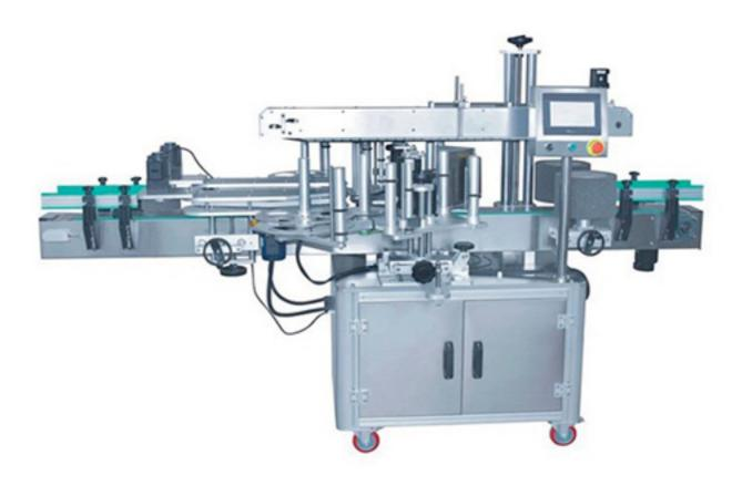
AR-60 Automatic double-sides labeling machine is suitable to the medicine, the date, food industry etc cylindrical container or small the conical taper container of ChanBiao, double standard automatic positioning labeling. This machine expanding strong! Can be equipped with all kinds of printer to print, online real-time can use single, also can use connect Product line.
