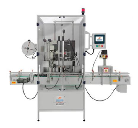
The Automatic Shrink Sleeve Label Applicator Machine consists of main structure, product transmission belt with guide adjustment, in-feed screw, sleeve former (mandrel), rotary cutter to cut sleeve, Safety acrylic cover, shrink tunnel with cooling fan, motors, sensors, electrical panel, AC drive, PLC & HMI.
