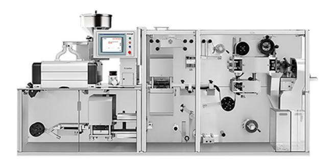
HM 300P is a blister packaging machine in an intermittent platen sealing motion with single lane mode of operation. This model is suitable for small and medium sized production, in which is capable of producing up to 300 blisters per minute. HM 300P is optimally designed for products with frequent size changeovers while ensures the greatest performance and quality for its price range.
