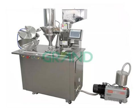
Capsule filling machine semi automatic is very compact and dynamic equipment to fill powder, granule, pellet into hard gelatin capsule in small scale, the filling speed is 200-300 pieces of capsule per min, as per the operation speed of operator.
