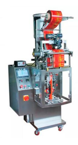
KST-300K packing machine can pack small granules of food, medicine, daily chemicals, tea, seed and some other material automatically. It has three pairs of rollers and can seal the package for three side or four side. Equipped feeder can also work for material to be packed in double sachets.
