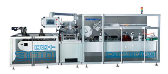
DZH-300 High Speed Continuous Automatic Cartoning Machine is a new design type of High speed great station automatic box packing machine. It is suitable for medicine blister, pillow pack, tube, bottle, ampoule bottle and similar goods. DZH-300 High speed cartoner adopt continuous transmission, synchronization pushing and rotary suction box device, the speed is faster and more smooth, less noise. Use the balcony type pushback layout, operation more convenient and clean up.
