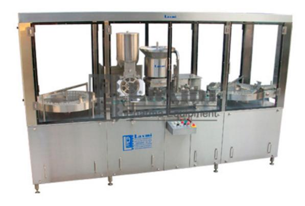
Laxmi Automatic Injectable Powder Filling & Stoppering (full & half bunging) machine. The basic unit consists of one or both side Turn Tables, S.S. Slat Conveyor Belt, Unique Powder Wheel. The machine is and can be run totally through Touch Screen HMI, PLC Control and the machine is based on servo motor drive, the machine has an output speed range of 80-240 vials per minute but depending upon the fill volume and container dia./size or the quality of powder.
