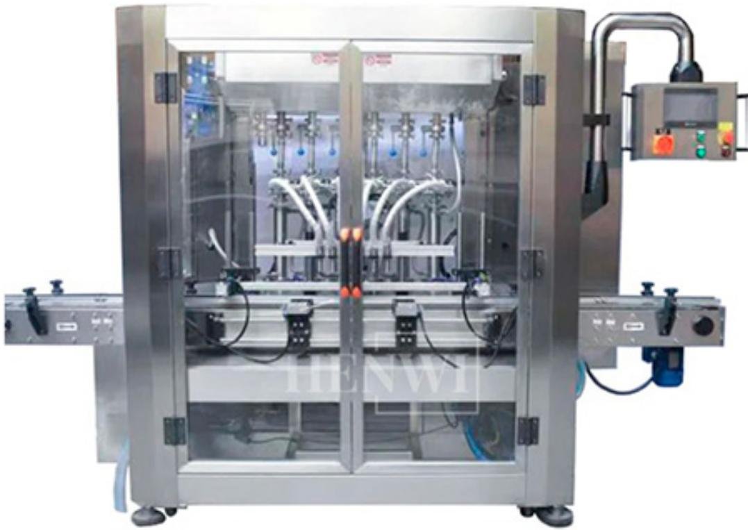
The automatic constant temperature servo piston filling machine is a highly advanced filling system designed for precise and consistent dispensing of various liquids, pastes, and high-viscosity materials. It is widely used in industries such as food and beverage, pharmaceuticals, cosmetics, and chemicals. Below are the key features, functionalities, and advantages of this machine.
