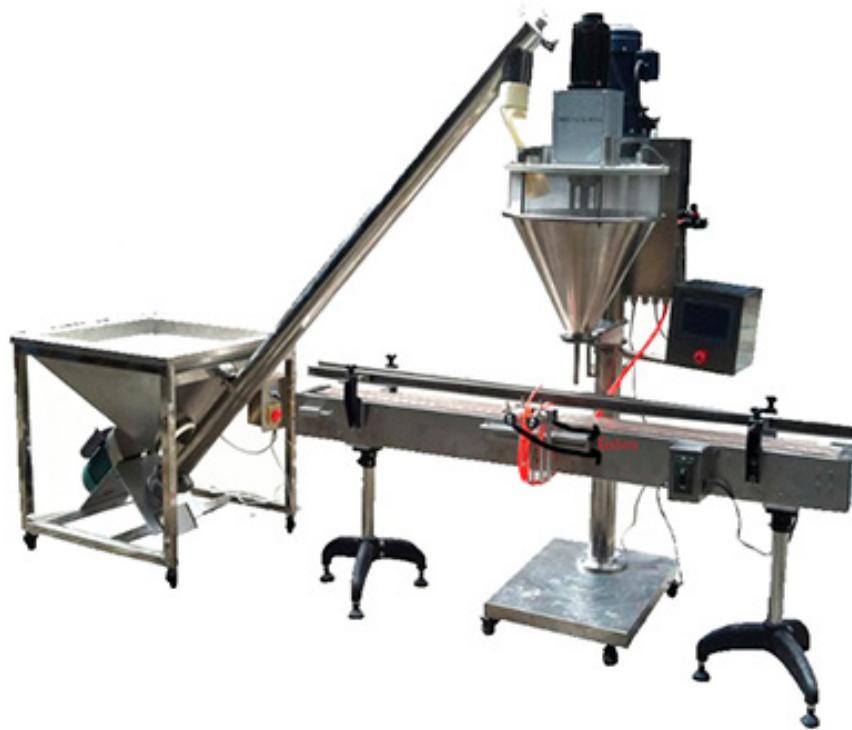
This line consists of bottle/jar feeding table, weighing filling machine, cap feeding machine, capping machine, labeling machine, etc. used for filling powder into bottle or jars.
