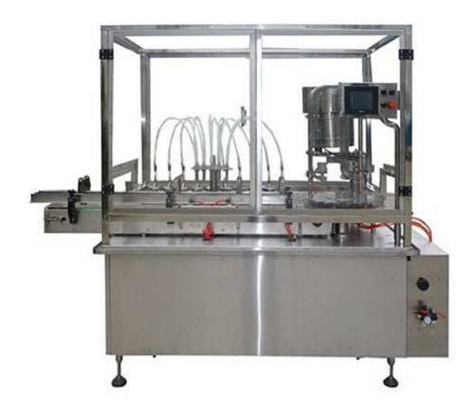
This machine is the main filling equipment of the vial production line, which is mainly applied in the filling, plugging, covering and capping of the 10 - 100 ml vials. This machine combines filling and sealing, advanced design, compact structure, the Replacement of the vial is very convenient.
