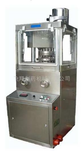
This machine is a single-press type; continue automatic tablet press for pressing granular raw materials into tablets. It is mainly used in pharmaceutical industry and also the chemical, food, electronic, plastic and metallurgical industries.
