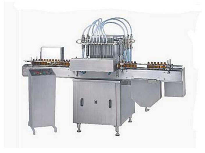
Working on volumetric principle, the unit is made compact, versatile and enclosed in stainless steel elegantly matt finish body.
