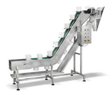
Applicable for lift-conveying of solid, granular, small-sized products, and more often for secondary lifting solution due to field space limitation.
