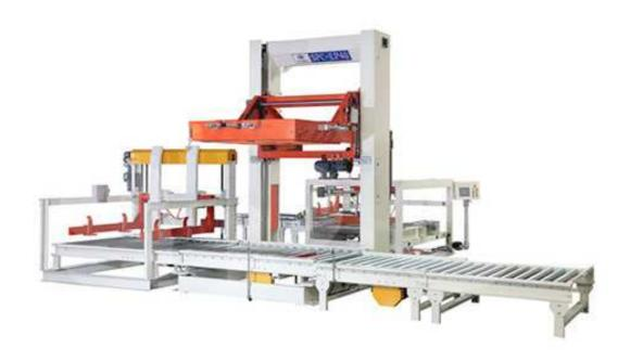
The palletizer is suitable for stacking carton, plastic case, shrink wrapped product and five gallons bottling etc. It consists of Case infeed, classification yard, pusher, pallet feeding etc. Optional interlayer keeps the stack more stable. It can be designed for different palletizing requirements with capacity ranging from 24000 to 72000 BPH.
