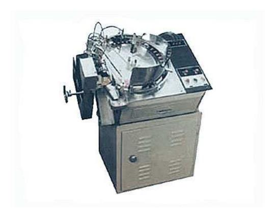
Feed disc and gravure rolls need to be changed to suit the shape and size of the product. Feed discs can be ordered with different numbers and sizes of pocket and can be interchanged in 5 minutes. Gravure rolls can also be ordered with any imprint and these are matched with the pocket spacing on the feed disc. Roll changing requires just one minute.
