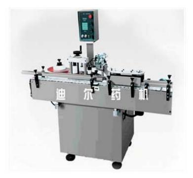
Description: This machine is used to stick mark circumferentially to column-model vessel, it is a mating product of ZP-I type omni-auto-counting and bottling line of pill, tablet, soft and hard capsule of our company, it can be used stand-alone and also can be used other matching product line.
