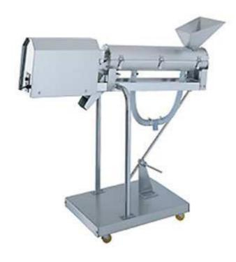
This polishing machine is used after capsules are for cleaning the powder attached on the capsules surface, through mechanically rotating brush and attraction of vacuum to take out the external powder of capsules.
