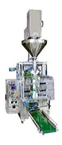
The MK-404 is a vertical form, fill and seal packaging machine designed to package various sticky powdered products. This VFFS packaging machine equipped with auger dose operates with electromagnetic clutch and it uses auger filling system to produce center sealed pouches also commonly known as pillow pack or fin seal type pouches / bags.
