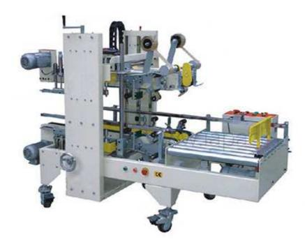
ZTF-400L Carton Sealing Machine is a flap folding carton sealer is easy to operate and maintain. Equipped with top bottom-side driving system, it can seal the carton top cover and carton bottom cover at one time, and sealing speed can reaches up to 25 cartons per minute.
