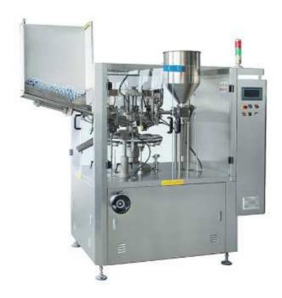
Aluminum Tube Filling Machine can be used in the industries of pharmaceutics, foodstuffs, cosmetics, daily chemicals for smoothly and accurately filling all kinds of pasty and viscous fluid and the materials alike, into metal tubes and then carry out tube end folding, sealing and lot number embossing.
