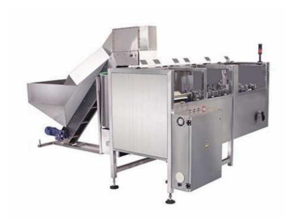
Randomly oriented bottles are received in bulk into the hopper and supplied to the centrifugal disc by means of a conveyor. In the disc, the bottles are guided into a qualified position suitable for the stand up unit to process them into the required discharge position Symmetrical bottles are stabilized and released on the customer conveyor.
