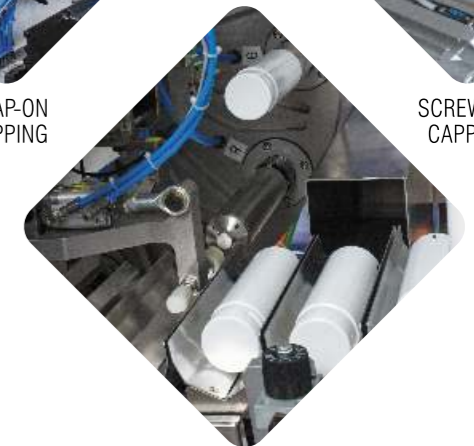
TUBE UNLOADING STATION
