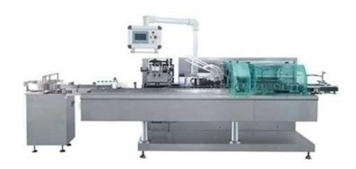
This machine is suitable for automatic feeding bottle (round, aquare bottle) into carton (either for blister or bottle). On line bottle unscramble and feeding, leaflet fold (1-4folds) and feeding, carton opening and forming, products and leaflet pushing into carton, printing batch number, sealing carton with tuck-in or hot melt glue device. Automatically reject lacking of leaflet or product and finished product out.
