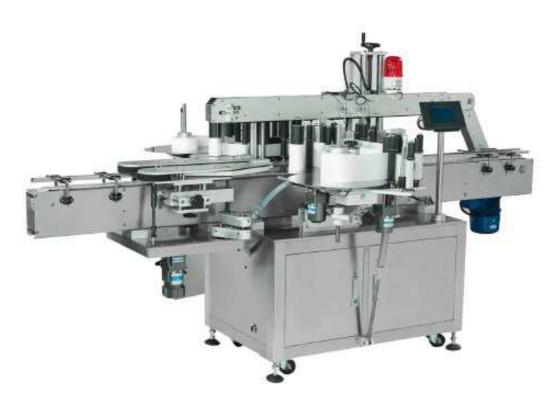
This Adhesive labeling machine used for food, medicine, cosmetics, electronics, hardware, auto parts, stationery, batteries, all kinds of bottles, and a variety of different specifications of the packaging products, automatic labeling machine work.
