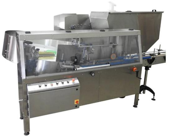
Automatic Bottle Unscrambler – Model TruSort-60 is capable of feeding and orienting plastic and metal containers.
