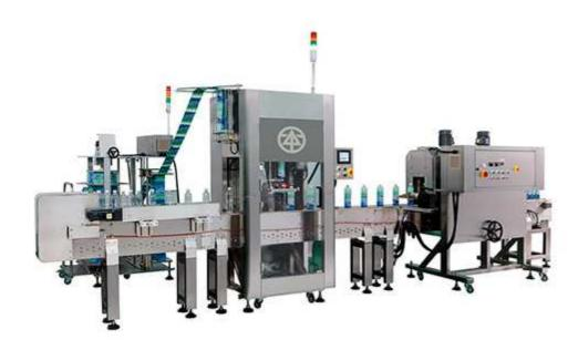
Auto Body Label Sleeve Applicator, LV-150 is designed with SUS frame to match production requirement of Foods & Pharmaceutical industries.
