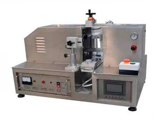
This ultrasonic tube sealing machine is widely used in pharmaceutical, cosmetic, food and chemical industries etc., it is applicable in various aluminum plastic compound soft tube, plastic soft tube which pack all kind of Such as ointment, adhesives, AB glue, Neoprene, epoxy glue, skin cream, hair cream, boots oil, toothpaste and else liquid, lotions and cream etc.
