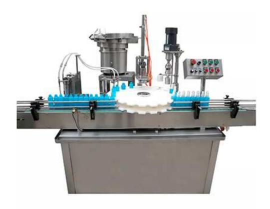
The Spray Filling Capping Machine is applied for liquid filling, automatically caps loading and screwing of bottles with long and thin pipe caps in pharmaceutical, food and cosmetics. The machine can automatically finish the bottle filling, bottle capping. With no bottle no filling feature.
