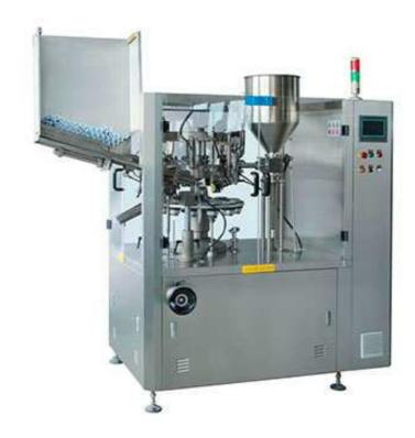
This machine can be used for filling cream and liquid materials, and it is characterized with firm filling and high precision of dosage. The three functions of filling, sealing and batch embossing can be completed automatically. It's widely used in pharmacy, daily chemical, food, chemical industries, (e.g.) pharmacy cream, hair color, toothpaste, leather oil, glue, nanp-epoxy adhesive etc.
