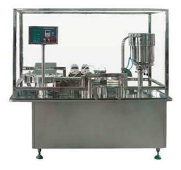
This liquid filling and plugging machine can be used for filling and plugging a wide range of glass bottles. Peristaltic pump and plunger pump have been used for filling work, and it can effectively prevent broken bottles from filling.
