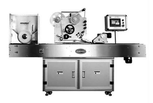
This blood collection tube labeling machine is used for 13\*75mm, 13\*100mm, 16\*100mm blood collection tube high speed labeling process. It applies PLC control for tube dropping, step-motor for label transporting, photoelectric detection for labeling and tube checking. This Blood Collection Tube Labeling Machine can be your most practical and economical choice without compromising on its performance and quality.
