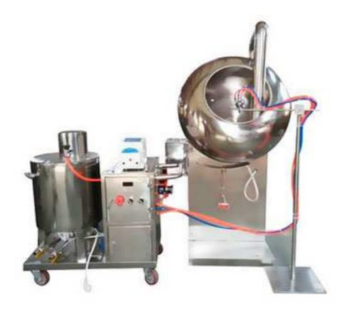
This machine is used to carry out sugarcoating and film coating to the core of Chinese traditional and Western medicine tablets. It integrates strong power, weak power, hydraulic and pneumatic. It is new type equipment improved on the basic of original common type sugarcoating machine.
