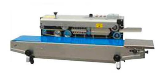
Band sealers are suitable for sealing individual pouches/bags automatically. The machine has a variable temperature controller and speed control, to suit different grades of plastic materials. Three types of models are available Horizontal type, Vertical type with foot stand type. Other special models include Nitrogen filling attachment, vaccum option, Printing attachment, and for heavy bags sealing
