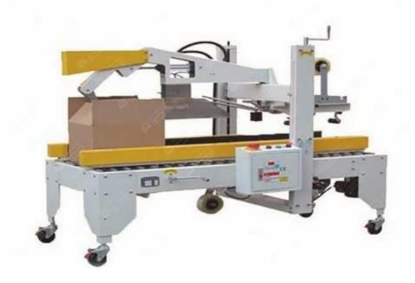
Fully automatic carton sealing machine mainly cooperates with the automatic production line, automatically folds the top cover, and the side belt drives the upper and lower seals. By adjusting the height and width of the machine, it can handle different sizes of cartons.
