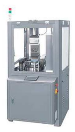
Total output of 6 000 filled & sealed capsules per hour. Designed for ease-of-use & high-precision. With the ability to quickly clean & change capsule sizes when needed. Versatile & reliable
