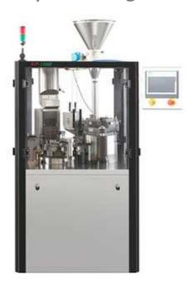
NJP-1200D Automatic Capsule Filling Machine adopts butterfly valve-type powder feeding, and is very suitable for drug powder with poor liquidity, including Chinese herbal medicine and Chinese patent drug, due to that its vibration unit equipped will force the powder to run down, which has solved problem of failing to feed in powder that often happens in the traditional screw feeding device because of the poor liquidity of powder.
