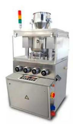
This machine is a new generation product which is developed from the former ZP45 tablet press of our company. It is a double-press type, continuously automatic rotary tablet press for pressing tablets. It is widely applicable to industries such as pharmaceutical, chemical, foodstuff, electronic and etc for pressing the granular material into all kind of round tablets, irregular tablets, two colors tablets and ring shaped tablets.
