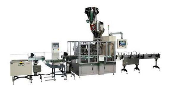
This Auger filling system provides a capability to fill a container at high speed by combination with a Rotary conveyer. The maximum speed would be 200 fillings per minutes. It is also possible to build up a high accuracy filling system by adding a correction filling station after the initial filling. There are variety of optional devices to make your complete production line, such as container feeding, capping machine, labeling machine etc.
